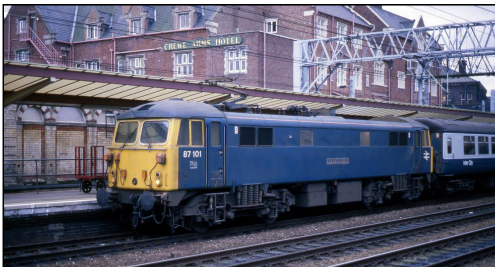
The first thyristor control locomotive on BR was built at Crewe in 1974 and used as an experimental loco until Jan.1977 when it entered public service. The name 'Stephenson' was transferred from 87001 (which became 'Royal Scot') in Oct.1977. The unique 87101 'Stephenson' is seen here at Crewe on 15 th January 1989, carrying its original stainless steel nameplates. photo: Paul Bettany
