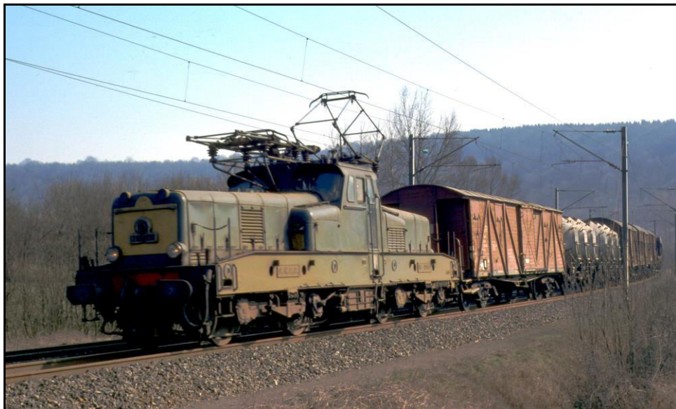
SNCF BB 12000, built in 1954 for operation on the 25kV Charleville line, still at work in northeast France in April 1976. Perhaps the ugliest electric loco ever built. photo: Jean-Claude Delagarelle.
