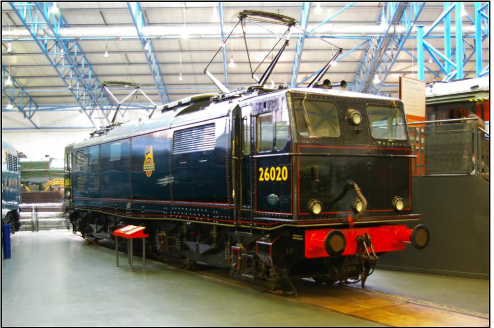
BR electric loco type EM1 Bo+Bo no.26020, built at Gorton in 1951 for the 1,500V DC Woodhead route electrification. On display at the NRM York. photo: Bob Gellatly
