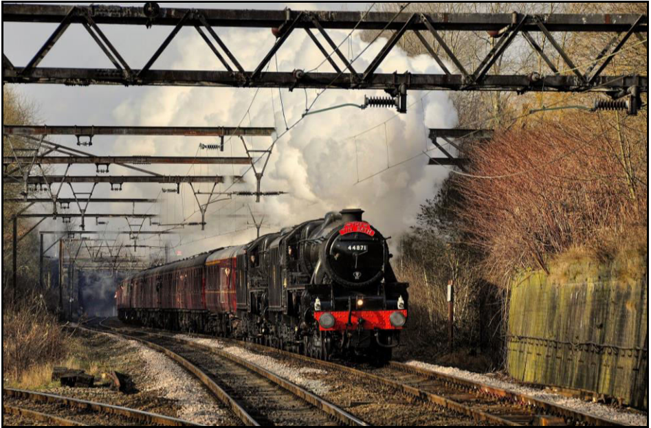
above: At the fourth attempt! "The Tin Bath" ran on 15 th Feb. 2015 behind Black Fives 44871 and 45407, seen here approaching Guide Bridge. The single track to Stockport is branching off to the left. The catenary supports date from the Woodhead scheme although the wires now carry 25kV AC current. photo: Anthony Roberts
